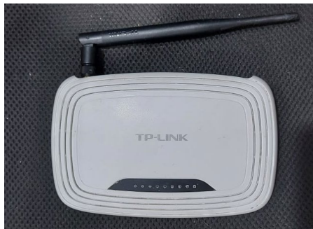
Figura 22: Router TP-LINK WR741ND.
