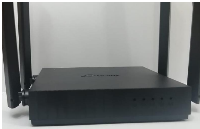
Figura 31. Router TP-Link AC1200 – Archer C54, leds indicadores.
