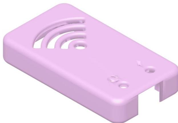
*Figura B. 2 Tapa Superior Carcasa ESP-8266*
