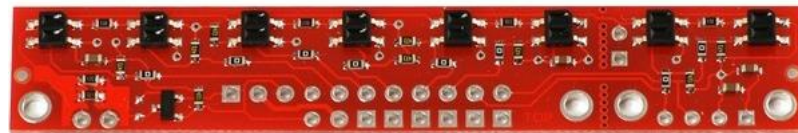
Figura 2.15 Sensor QRT8A Pololu. (Pololu Corporation, 2021)
