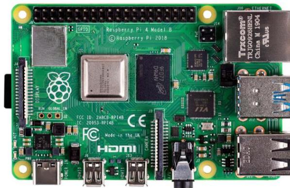
**Figura 4.** *Raspberry Pi 4 Computer Model B*
