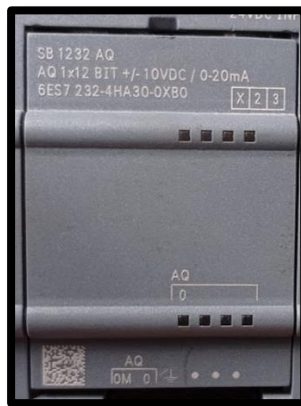
Figura 25 Signal Board SB 1232 AQ (Salidas digitales)
