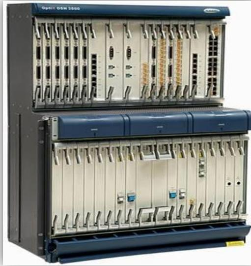
**Figura 2.m.**Multiplexor Huawei OSN3500
