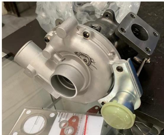
***Figura 10*** Turbocompresor RHF4H
