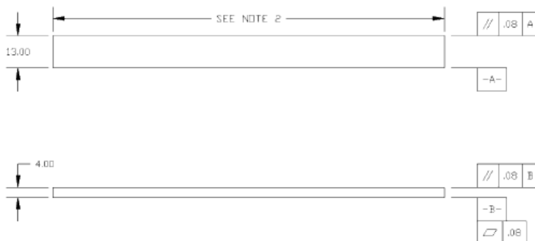
FIG. 4 Standard Flexural Test Specimen Drawing (SI)
