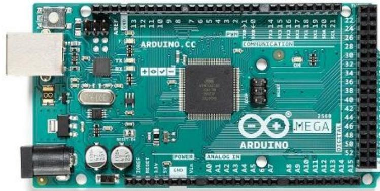
Figura 3.8 Arduino Mega 2560. (Arduino, 2020)
