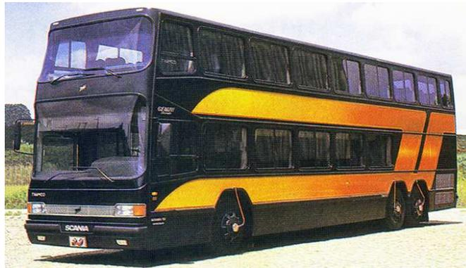
**Figura 5.** Gemini Thamco DD en chasis Scania K-112TL
