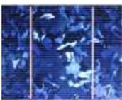
A rectangular solar cell with a blue, multi-colored, and textured surface and two vertical silver lines. | 12...14%   | Estructura cristalina no uniforme. Se fabrica en moldes rectangulares. Menor coste que el silicio monocristalino.                                     |
