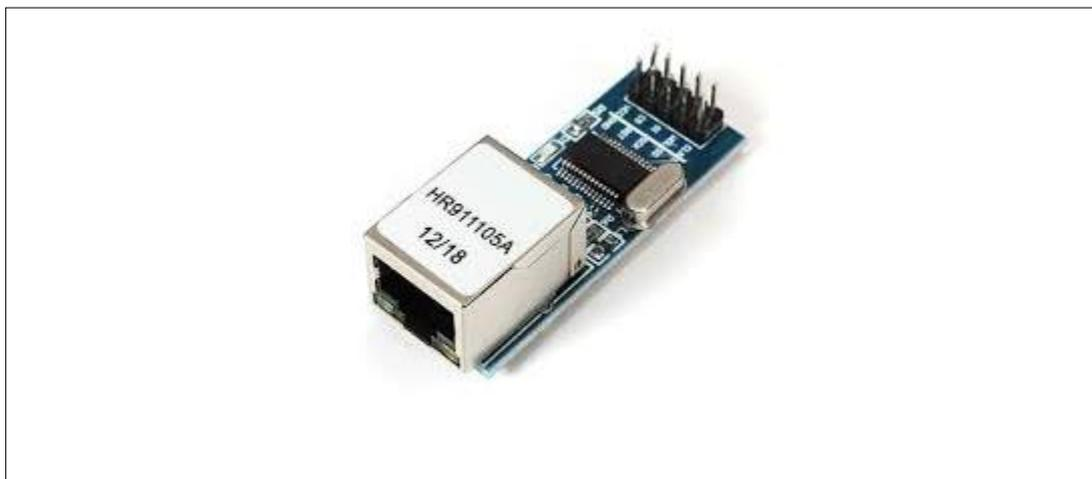
*Figura 9: Shield Ethernet. [24]*
