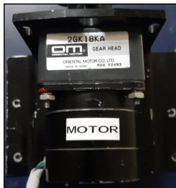
Figura 2.21 Caja reductora 2GK18KA
