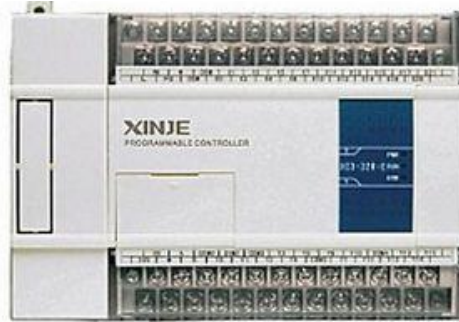
Figura 3.16 Automata Programable XINJE XC3-32RT-E
