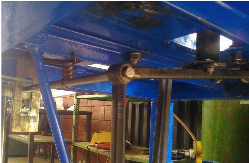
**FIG. A4.10 SISTEMA DE FRENADO**
