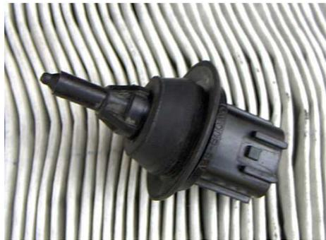
**Fig. 1.12 Sensor IAT (Intake Air Temperature)**
