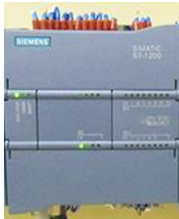
Figura 3-5 PLC S7-1200 1212C AC/DC/RLY
