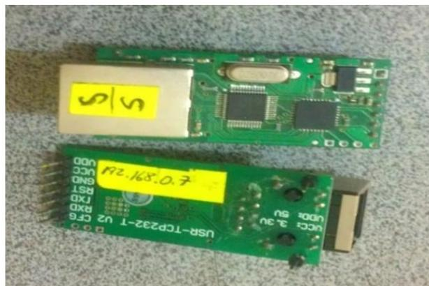
**Figura 2.35** Convertidor Serial a Ethernet Por: Wave share Electronics, (2013).
